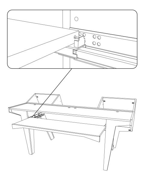
To secure, push the keyboard tray until the front latches engage and click into place.
