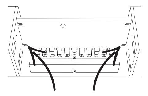
Secure the 2 interior fasteners before determining the monitor shelf orientation.
